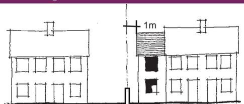
**DO** have a minimum distance separation between a common boundary and any new extension. A minimum 1m distance from the common boundary and any wall of a new two storey extension should be provided. Single storey extensions may be built up to the boundary.
