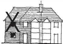
DONT change the traditional compositional balance of the semi detached dwelling by introducing a new extension that runs continuously from the existing roof or wall line.
